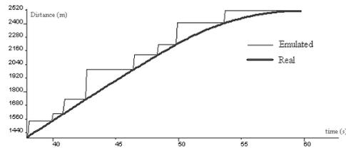
Fig. 2. Rejected takeoff distance emulation
